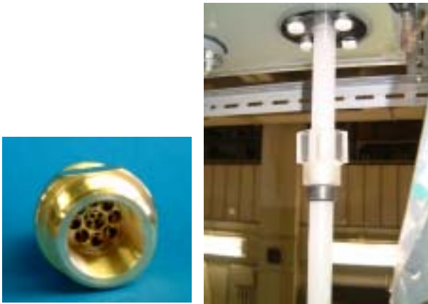
Fig.3 Cavitation nozzle and milky bubbly flow
