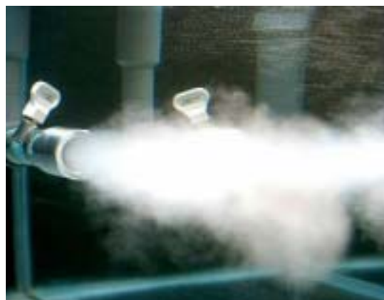
Fig.2 Micro bubble generation by cavitation nozzle
